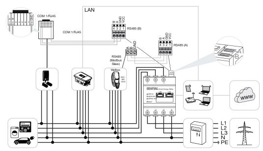
Only one KOSTAL Smart Energy Meter is required to monitor power and limit feed-in at the grid connection point. This is installed at the grid connection point in the house grid as shown in the illustrations.
